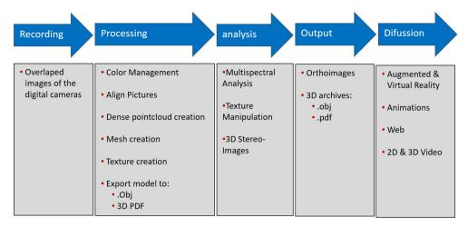
Fig. 5. Photogrammetric Processing Stages.
