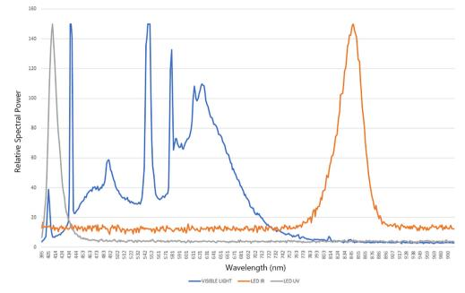
Fig. 3. Spectral signatures of lights at working distance. The vertical axis represents the Relative Spectral Power measured and the horizontal axis the wavelength in nanometers where it was measured.
